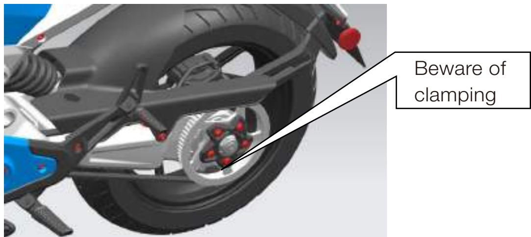
Image1 Dangerous area of sprocket
