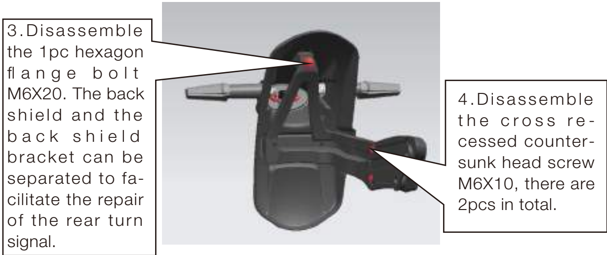
Image 30 Disassemble the rear license plate bracket
