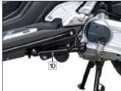
7. Side (10) switch at horizontal position.
