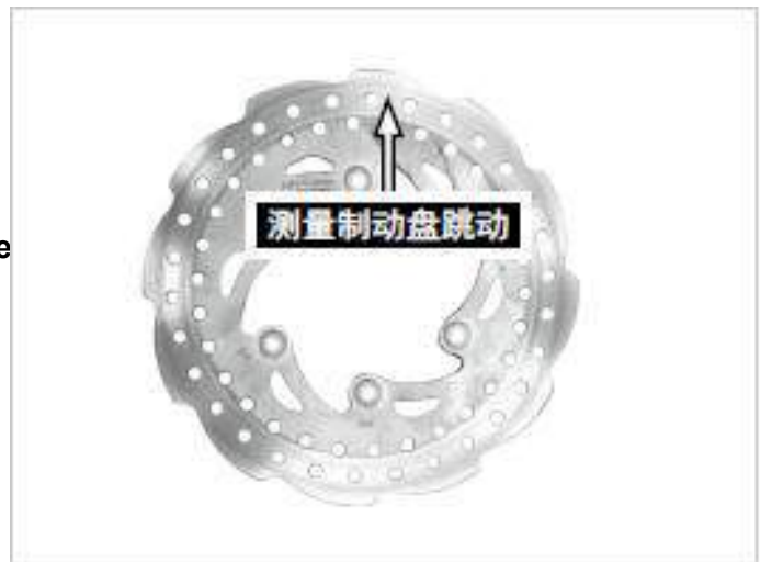
Measure the brake disc runout
