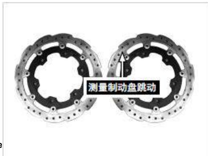
Measure the brake disc runout
