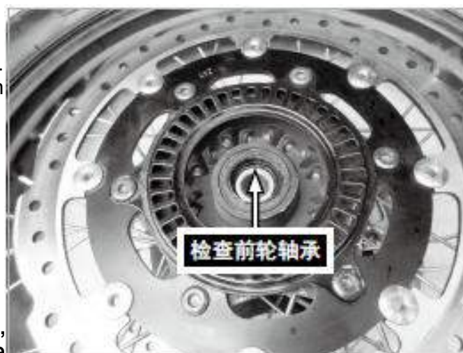
Check front wheel bearing
