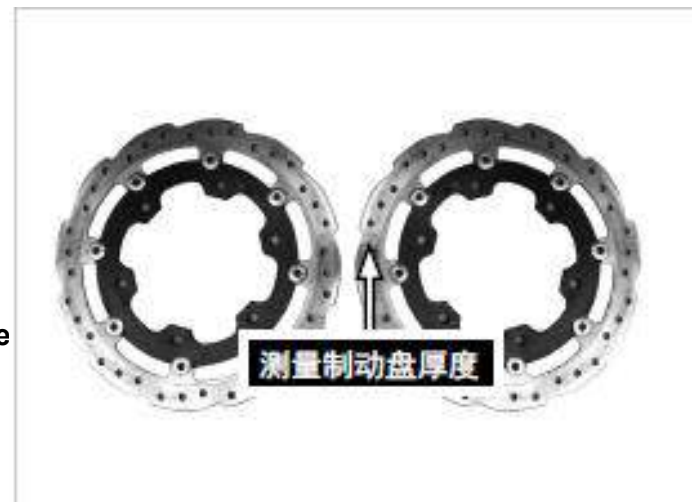
Measuring brake disc thickness
