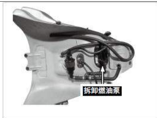
Removing fuel pump
