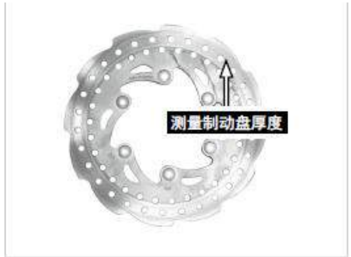
Measuring brake disc thickness
