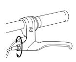
**1** To adjust brake cable play, thread the brake lever adjuster in or out 1/4 to 1/2 turn until the desired brake adjustment is attained. Most adjustments are complete at this step. If brake still needs further adjustment, proceed to step 2.
