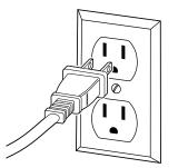
**1** Plug the charger into a wall outlet. The light on the charger should be green.
