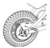
**1** Loosen screws and remove chain guard.
