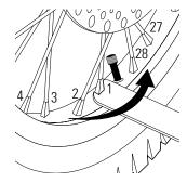
**2** Start with spoke closest to the tire valve stem and tighten each nipple, in sequence, exactly 1/4 to 1/2 turn. A single 1/4 to 1/2 turn may not be enough to bring the spokes into proper tension. Continue tightening all spokes, no more than 1/2 turn, in sequence until all spokes are tight.
