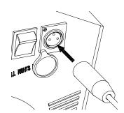
**2** Maker sure power switch is in the **OFF** position. Plug the charger into the charger port. The light on the charger should turn red during charging then back to green when charging is complete.
