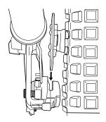
**1** Position wheel in front fork and slide disk brake into caliper.
