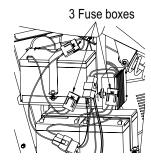
**1** Remove the seat fairing and battery cover to locate the 3 fuse boxes attached to the batteries.
