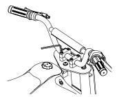
**2** Align parallel to the fork and tighten the bolts using a 6 mm Allen wrench. When properly tightened, the handlebars should not move forward or backward.
