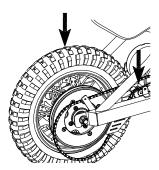
**3** Push the chain tensioner down to loosen the chain and remove the chain from the wheel sprocket and motor sprocket. Push and remove the wheel downward.
