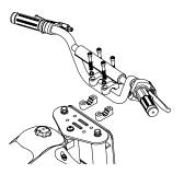
**1** Place the handlebars in the handlebar clamps with tools and manual.
