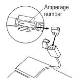
**2** Check all 3 fuses to see if the fuse(s) have burnt out. Remove any fuse that is damaged or burnt out and replace with a new one of equal amperage.
