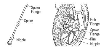
1 Verify the spoke tension by shaking each spoke with your fingers. Spoke should not be loose from hub. Look for any play between where the spoke flanges attach to the hub. Try to turn the nipple using your fingers. You should not be able to spin any nipple by hand. If one or more spokes is loose, all spokes must be checked and need to be tightened with a spoke wrench.
