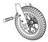
**1** Using a Phillip screwdriver, loosen the two (2) screws on the fork covers (2 per side) and remove covers.
