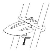
Align fender with the hole in the fork and insert the bolt. Tighten securely using a 10 mm wrench and 5 mm Allen wrench.
