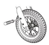
**3** Remove front wheel and install replacement wheel. Re-attach fork covers.
