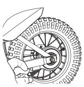
**8** Thread the brake cable through the brake adjuster barrel, through the large spring, and into the small hole in the side of the anchor bolt. Position the cable to the original location (as indicated by the slight cable kink) and tighten securely.
