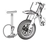
Using a bicycle tire pump equipped for a Schrader valve, inflate both tires to the PSI indicated on the sidewall of the tire. WARNING:
