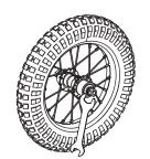
**2** Remove the nuts on both sides of the front axle using a 15 mm wrench then remove the axle safety washers.
