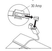
**6** Remove the fuse and replace with a new one of equal amperage. Close the fuse cover and reattach the battery cover, fairing, and plastic cap.
