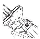
cap **2** Using a 5 mm Allen wrench, remove the bolt.
