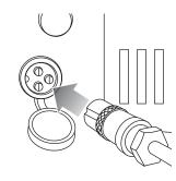
**2** Make sure the power switch is in the **OFF** position. Plug the charger into the charger port on the product. The light on the charger should turn red during charging. The light will turn green when the charging is complete.
