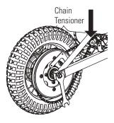
**4** With two (2) 15 mm wrenches, loosen the axle. Push the chain tensioner down to loosen the chain and remove wheel.
