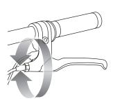
**1** To adjust the tension, thread the brake lever adjuster in or out 1/4 to 1/2 turn until the desired brake adjustment is attained. Most adjustments are complete at this step. If brake still needs further adjustment, proceed to step 2.
