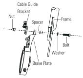
**7** Install the cable guide bracket to the frame and brake plate using bolt, washers, and nut. Do not tighten.
