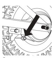
2 If the brake has too much slack, use a 10 mm wrench to loosen the brake anchor cable for additional adjustment and retighten.
