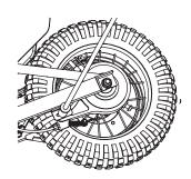
**3** With two (2) 8 mm wrenches remove the cable guide bracket from the frame and brake plate. Keep the spacer and washers together.
