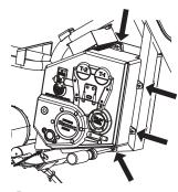
**4** On the opposite side of the charger port, locate and remove the five (5) Phillips screws and lock nuts on the battery cover using a Phillips screwdriver and 8 mm wrench. Separate and remove cover.
