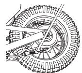
**9** Tighten the cable guide bracket bolt. Tighten the locknuts on the rear axle. Test the brake to verify proper function before riding. Readjust as needed.
