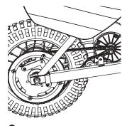
**6** Verify chain is properly installed on each sprocket and tensioner is correctly positioned at the bottom of the chain.
