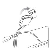
**5** Locate the fuse box attached to the batteries. Open the fuse cover to expose the fuse.
