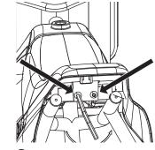
**3** Using a 5 mm Allen wrench, loosen the two (2) bolts underneath the rear of the seat and remove the fairing.
