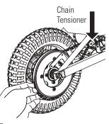
**5** Install the chain onto the rear wheel sprocket. Slip wheel axle into the frame slots. Push the chain tensioner down to create slack in chain. Hand tighten rear axle locknuts.
