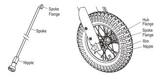
**1** Verify the spoke tension by grasping and shaking each spoke. Spoke should not be loose from hub. Look for any play between the spoke flanges where it mates with the hub. Try to turn the nipple using your fingers. You should not be able to spin any nipple by hand. If one or more spokes is loose, all spokes should be checked and tightened with a spoke tightener.
