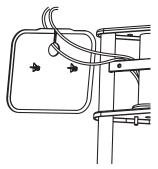
Slip the cables through the slit on the top of the number plate. Align the number plate with the holes on the fork and snap on the number plate.
