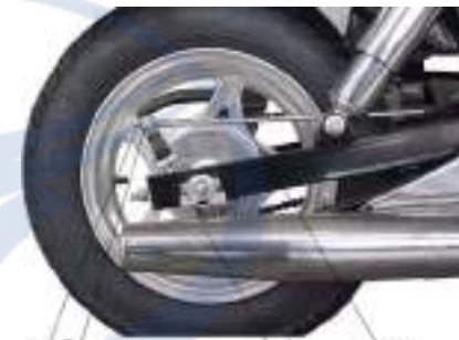
1 adjusting nut 2 brake arm pin 3 rear brake arm 4 brake pull rod
