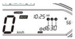
After setting the minute of the time, press the adjustment button again for a long time. The hundreds place ① of the front tire diameter will start flashing, and the short press will cycle between 0 and 9.
