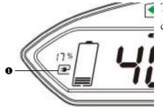
This charging indicator symbol **1** display when the battery is charging.
