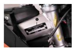
The nameplate **1** is mounted on the chassis at the front right.
