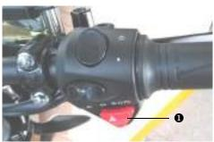
When the button **①** is pressed, the turning lights flash to warn other drivers of situations, which include stop or park under emergency conditions.
