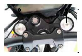
The hydraulic rebound damping system determines the performance of the front suspension when it bounces up. The adjusting bolt **1** is located at the upper end of the front suspension leg.
