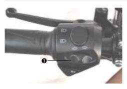
The steering lamp switch **①** is on the left handle switch. When the steering lamp switch is pushed in the left or right position, the corresponding
