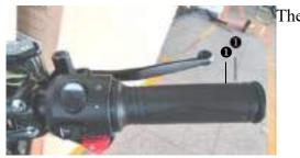
The throttle grip **0** is fitted on the right side of the handlebar.
