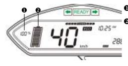
Display the battery capacity as a percentage.Display the battery capacity as an icon.
