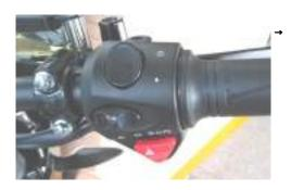
Select the driving mode switch on the right-hand handle switch. There are three modes for selection.
