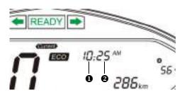
While the motorcycle is powered on, press and hold the adjustment button at the back of the instrument for 3s to enter the setting interface.
