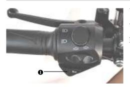
When the key is in the ON position, the horn sounds when the button **①** is pressed. the horn can be used to warn pedestrians or other motorists of your presence.
