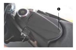
The charging dock is in front of the seat. Press the back of the charging cover to open it.
