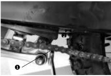
Push the chain at the lower end of the chain support **①** upward to check the tension of the chain between the chain and the chain support.
