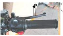
The front brake handle **1** is fitted on the right side of the handlebar.
