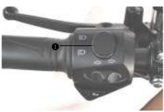
The headlight high/low beam **1** switch is on the left handle switch.
