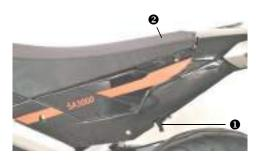
The seat/helmet lock is located at the rear left side of the motorcycle.
