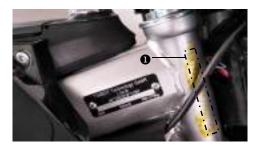
The chassis number **1** is stamped on the right side of the steering head.
