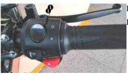
Flip the switch upward to 🖏, open the Headlight. Flip the switch down to •, open the Headlight.
