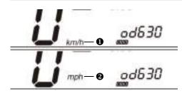
After setting the front tire diameter parameter, press and hold the adjustment button again to enter the MM/INCH setting. At this time, km / h① characters begin to flash. Press the adjustment button briefly and mph② character begin to flash, namely switching to INCH display mode.
