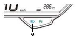
When the headlight high beam is on, this indicator **①** illuminates blue, and remains on until the high beam is turned off.
