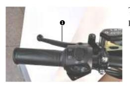
The rear brake lever **1** is fitted on the left side of the handlebar.
