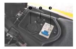
The main circuit breaker **③** is the protection switch of Ranger main power supply. When the current caused by abnormal or short circuit of the motorcycle exceeds the safety setting value, the air switch will be automatically disconnected to ensure safety.
