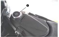
Start/stop button is used to start or stop the motorcycle.
