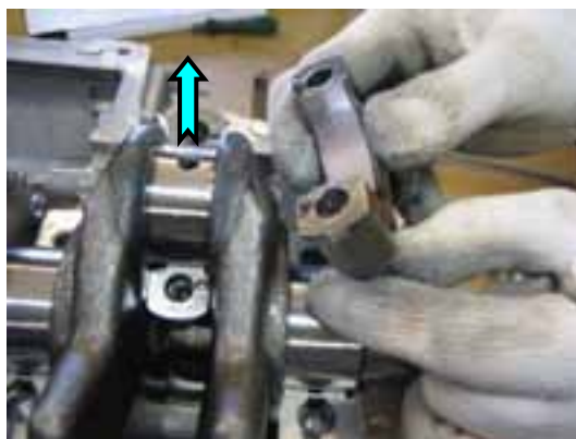
Remove the connecting rod cap , then remove the crankshaft
