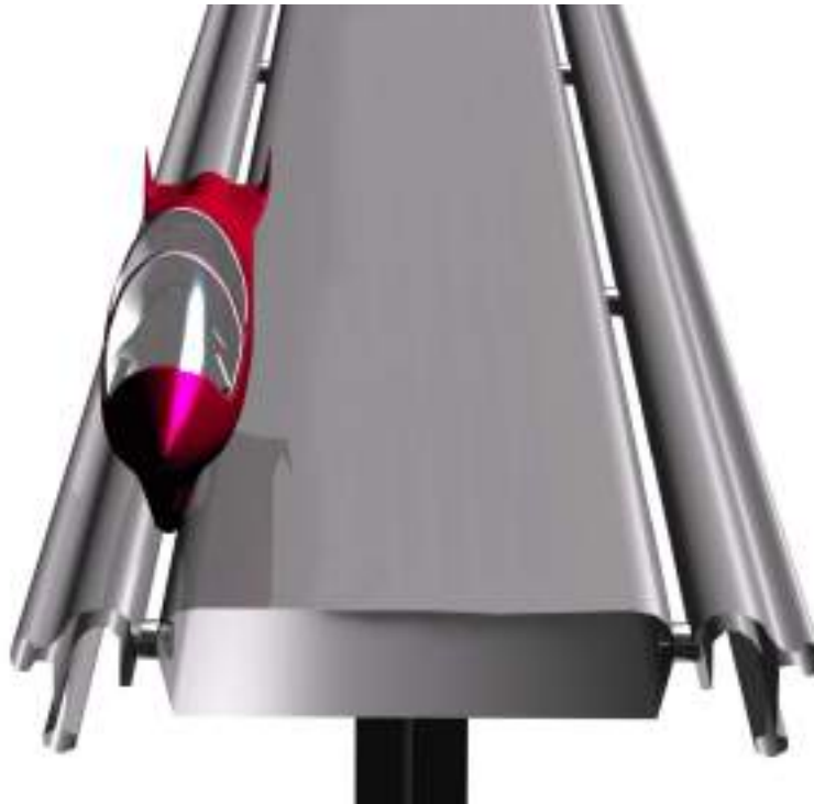
Fig. 18: V-shaped rail for secure driving even in extreme weather
