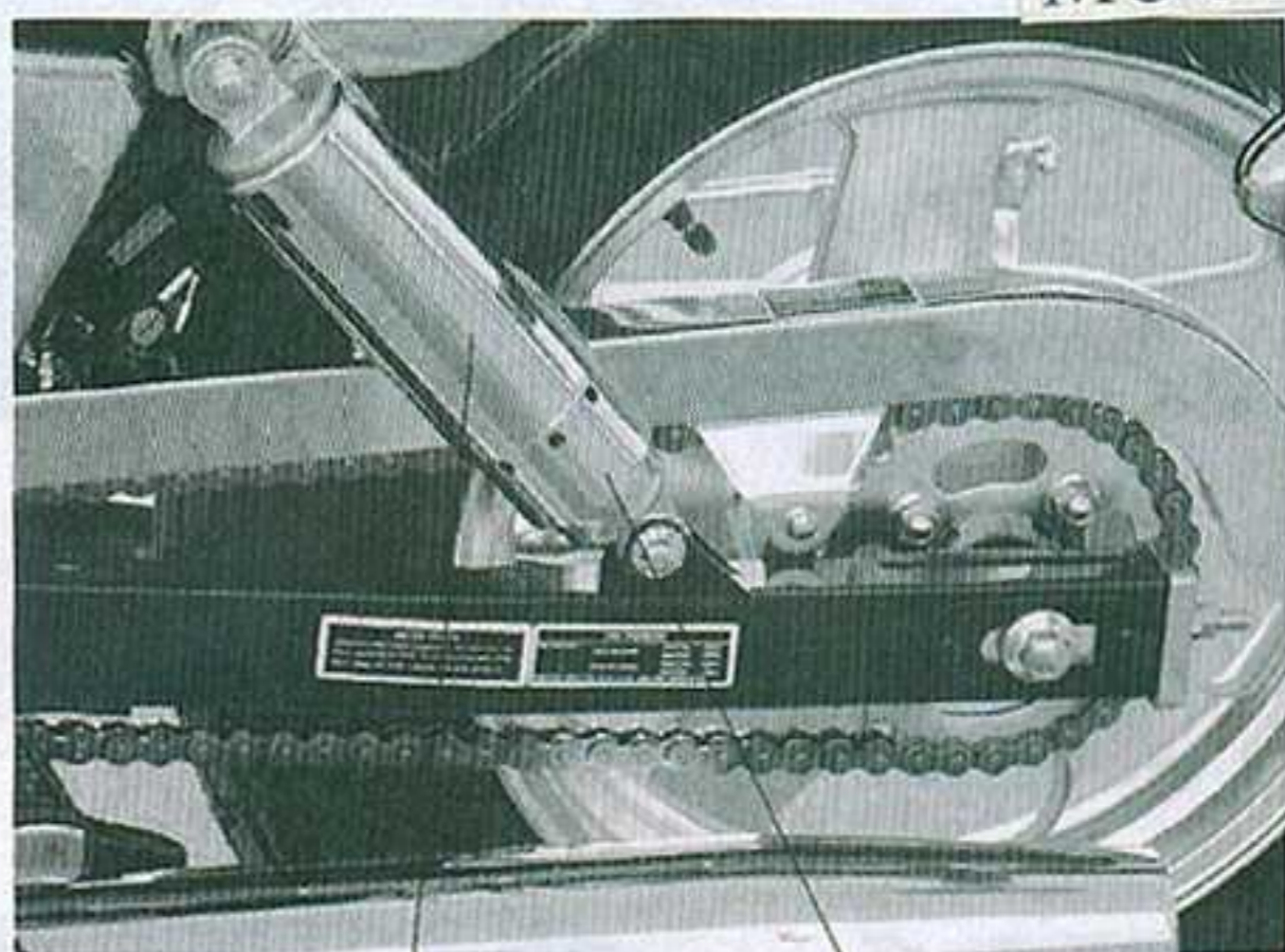
① rear shock absorber ②1~5 adjusting position marks
