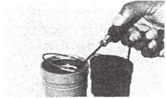
2. Remove the ring that holds the seal in place. Use a screwdriver.
