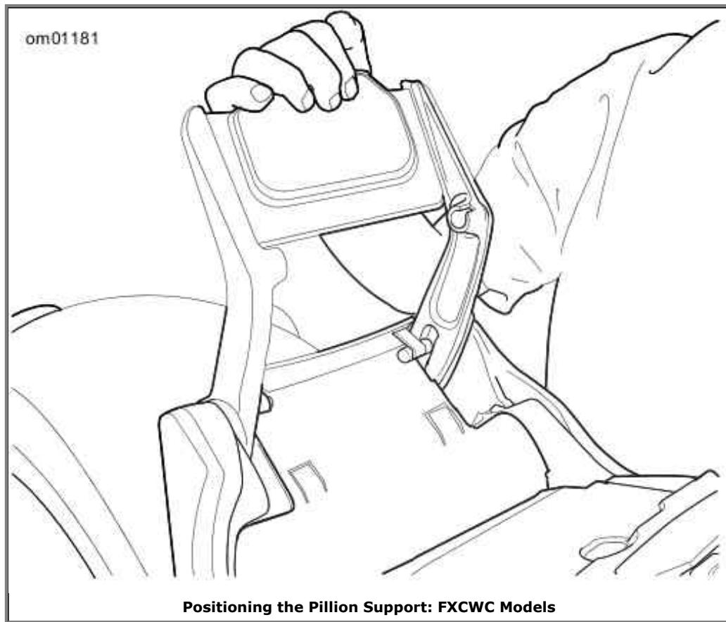
2. See Positioning the Pillion Support: FXCWC Models. Slide hinge pins of pillion support upward in side upright slots, then rotate pillion support approximately 180 degrees.
