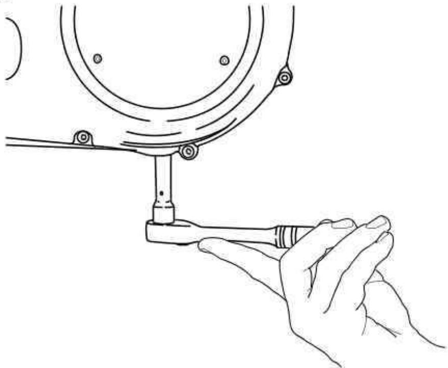
Removing Chaincase Drain Plug
