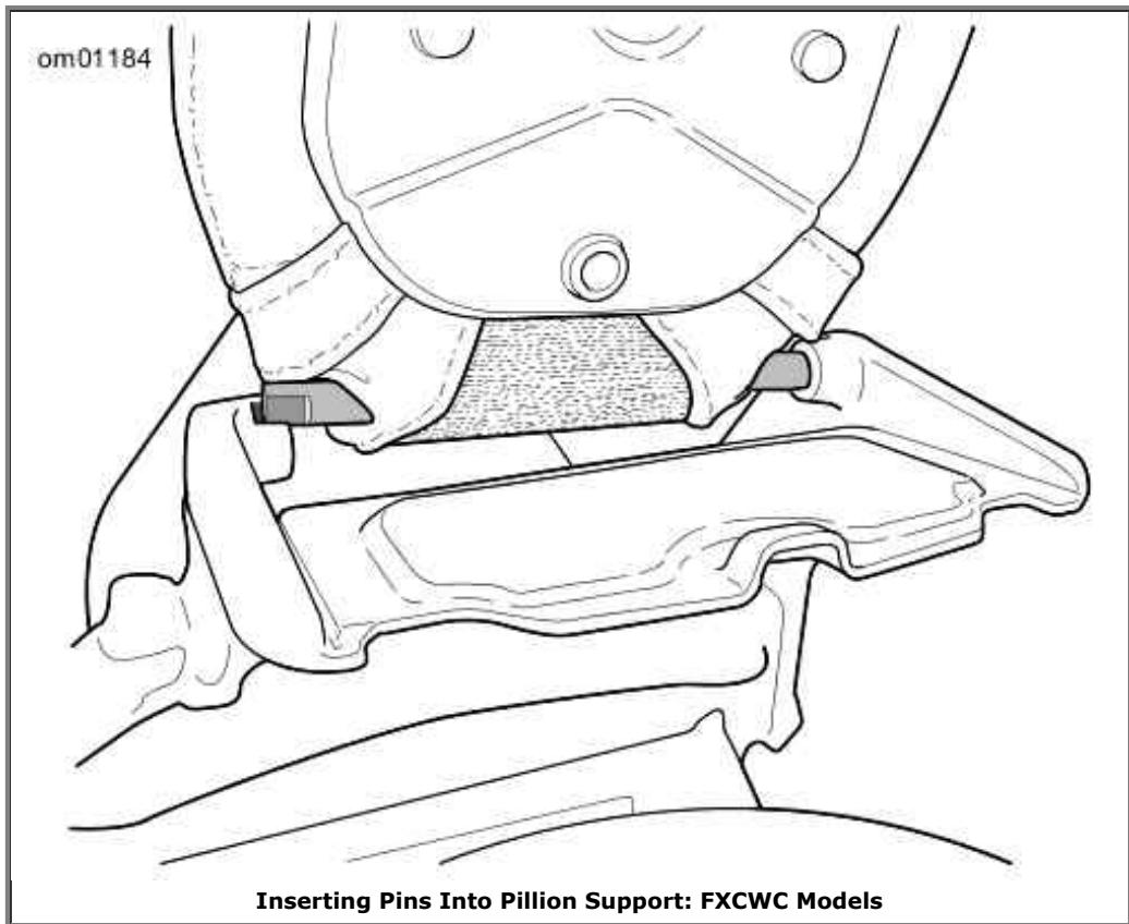
7. See Inserting Pins Into Pillion Support: FXCWC Models. When the pillion pad is approximately vertical, the left side flat key can then be put into its pivot seat on the pillion support.
