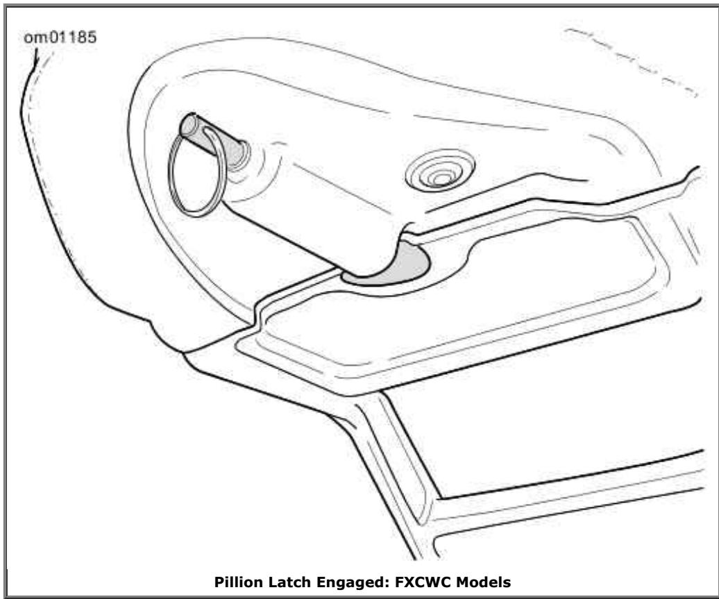
8. See Pillion Latch Engaged: FXCWC Models. Rotate the pillion pad to its horizontal position. Apply slight pressure on the end until the pillion pad latch catches on the back of the pillion support.
