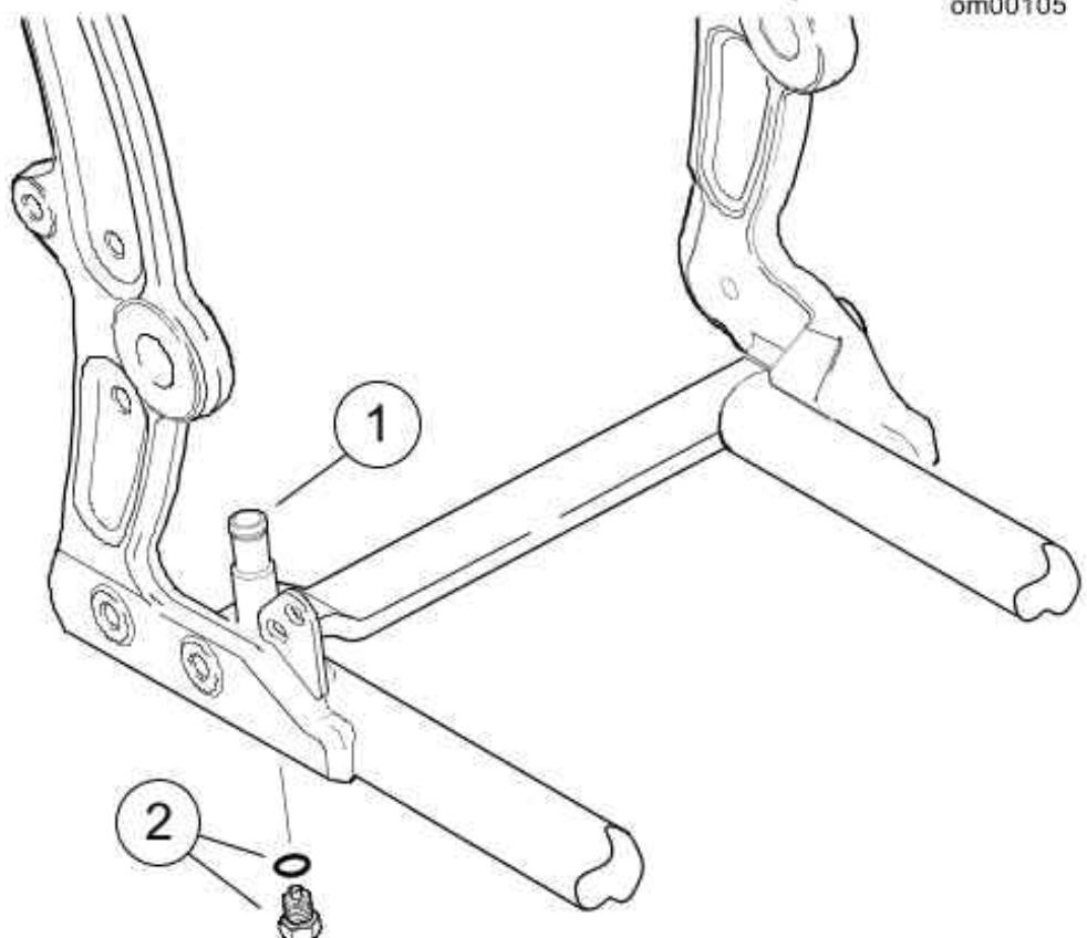
1. Frame connection for oil tank drain hose
