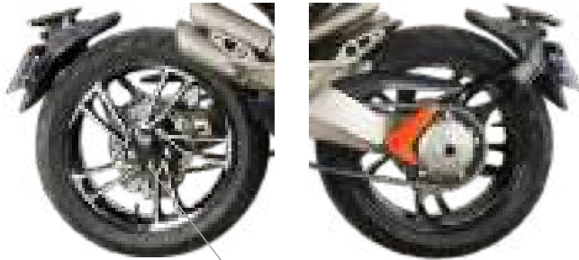
M12×1.5 nuts Rear wheel nut tightening torque: 110N.m
