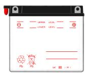
The vehicle is equipped with a maintenance-free battery. The battery is placed in the left side of the vehicle, protected by the battery cover. When put in or take out the battery, use key open the battery cover first.
