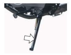
To use the main, depress it by foot and lift the rear of the motorcycle until the rear wheel is lift. To use the side, depress the end of it until it
