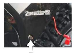
Above indicates the lock is the battery box protection cover, to take out the battery, please open the lock with a key switch.
