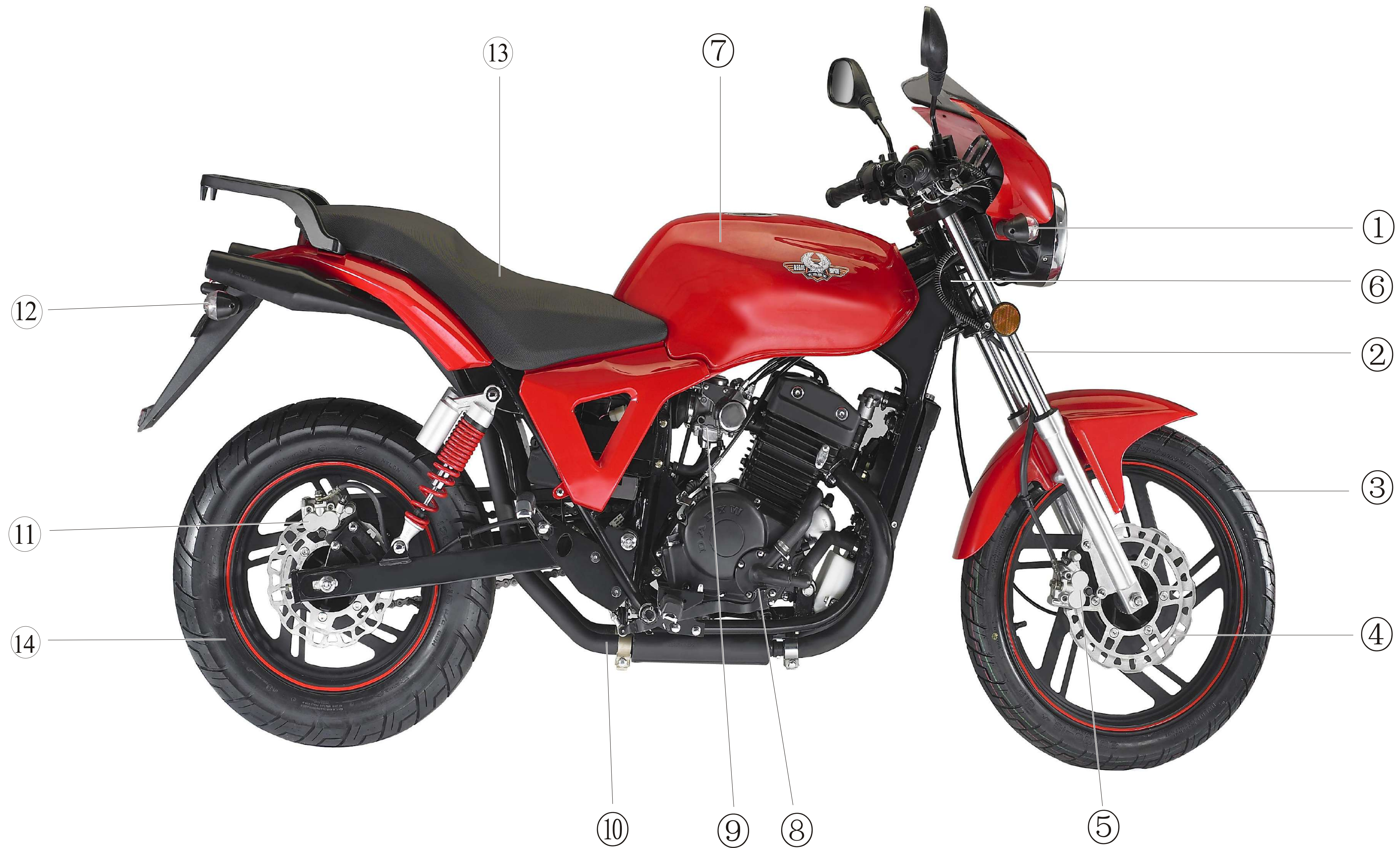
①Front right turn signal light ②Front Shock absorber ③Front wheel ④Front brake disc ⑤Front brake pump ⑥Frame name plate ⑦Raditor ⑧Rear Brake padel ⑨Carburetor ⑩Right muffler ⑪ Rear brake ⑫Rear right turn signal light ⑬Seat ⑭Fuel tank
