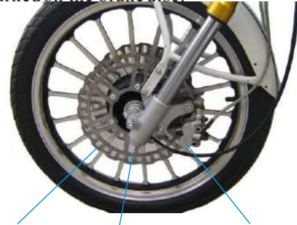
Brake disc Wear markleft (Left) Brake calipers
