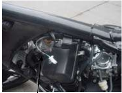
fuel sensor wiring
