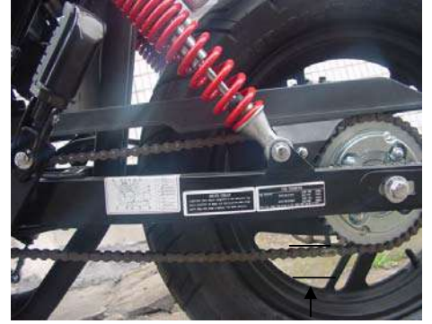
Chain tolerance: 15-25mm
