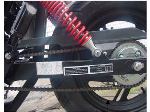
Chain tolerance: 15-25mm
