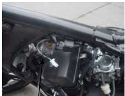
fuel sensor wiring
