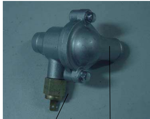
heat sensor thermostat hull
