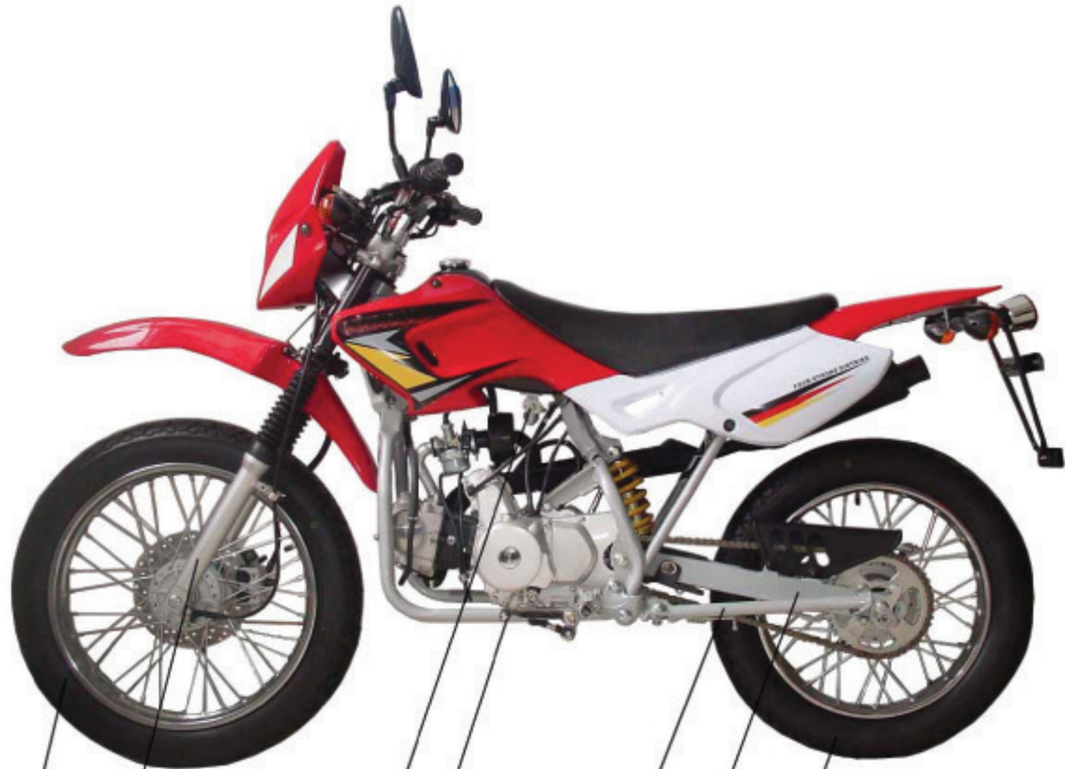
1. front wheel 2. front shock absorber 3. fuel tank 4. gear shifting 5. side stand 6. rear fork 7. rear wheel
