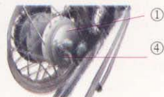
Fig. 34 ① Rr. brake panel ② Reference mark ③ Indicator ④ Rr. brake arm
