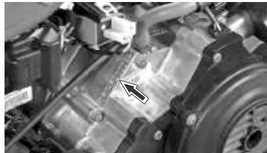
The engine serial number is stamped on the top surface of right side crankcase near engine breather tube.
