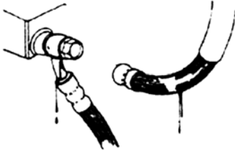
(leak, damaged, looseness of brake line)
