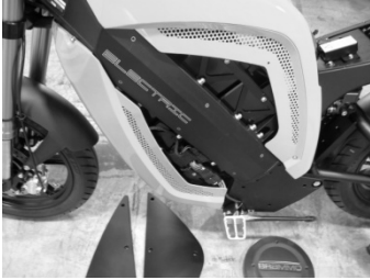
3. Remove the side panels
