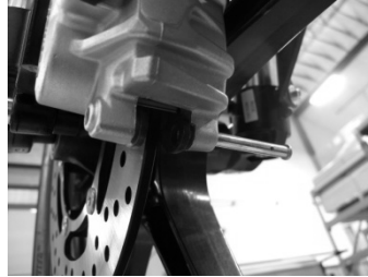
2. Remove the pin
