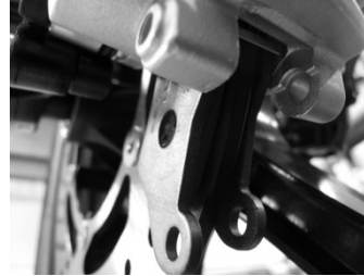
3. Remove brake pads
