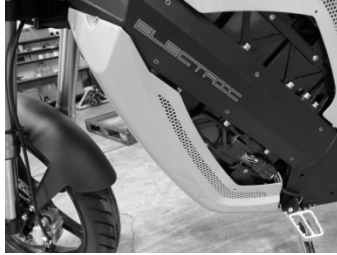
4. Remove the lower body panel
