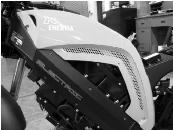
5. Remove the upper body panel
