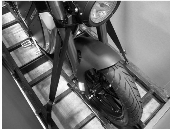
Using tie-down straps to secure your Enertia for transport
