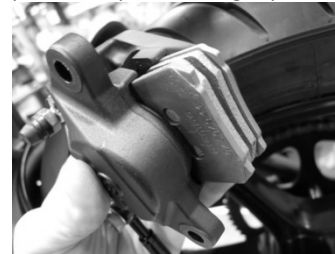
3. Remove brake pads
