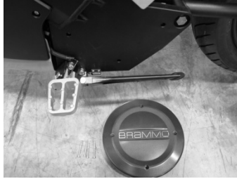
2. Remove the motor covers
