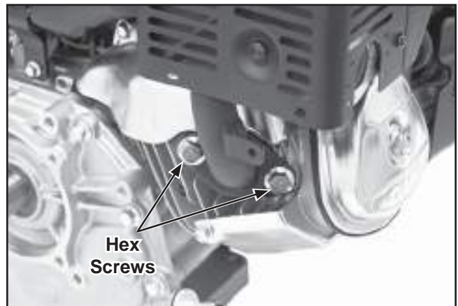
Figure 11-87. Install CH395, CH440 Muffler/Heat Shield Assembly.
