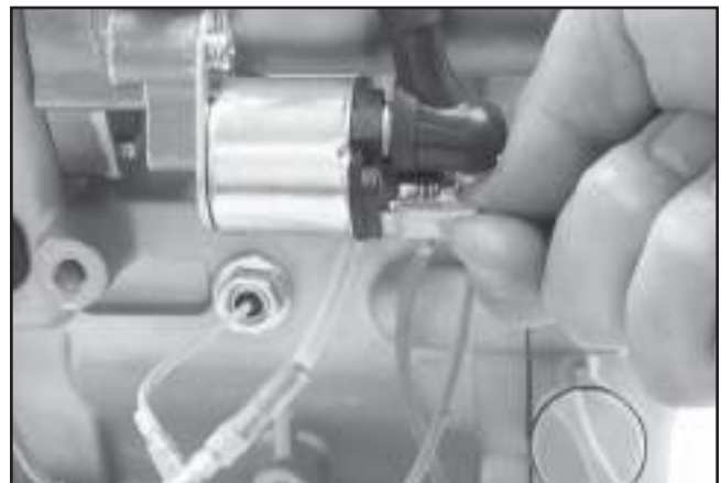
Figure 11-68. Connect Electrical Leads.
