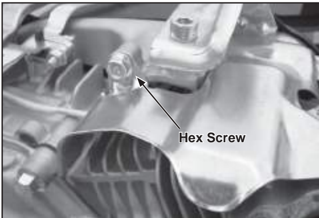
Figure 9-21. Remove CH270 Upper Shield Hex Flange Screws.
