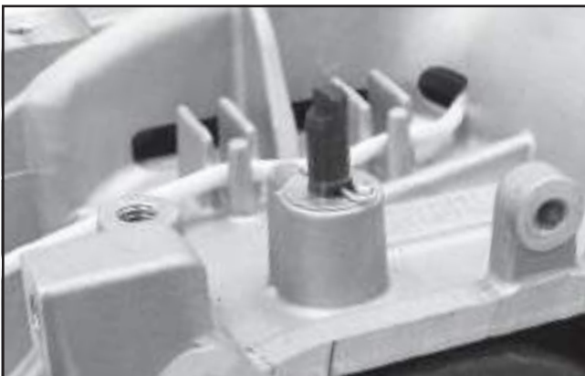
Figure 9-60. Removing Governor Cross Shaft Hitch Pin.
