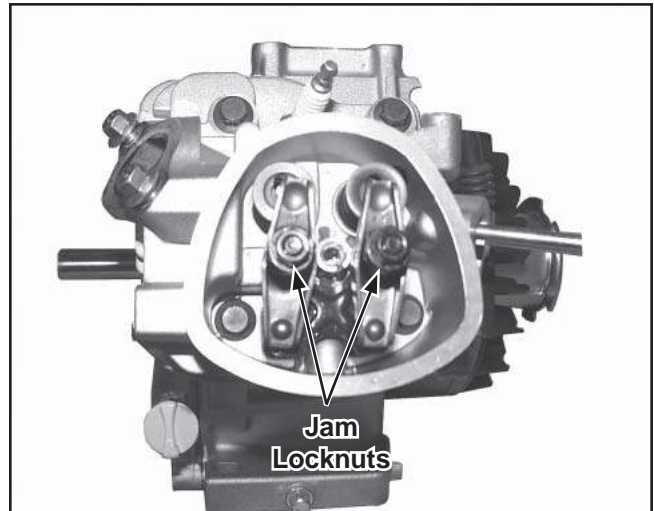
Figure 11-49. Installing Rocker Arms, Adjusters and Locknuts.
