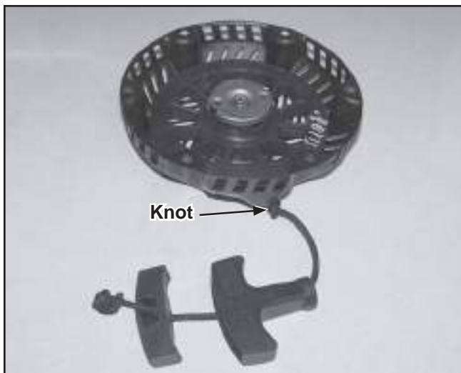
Figure 7-3. Removing Starter Handle.
