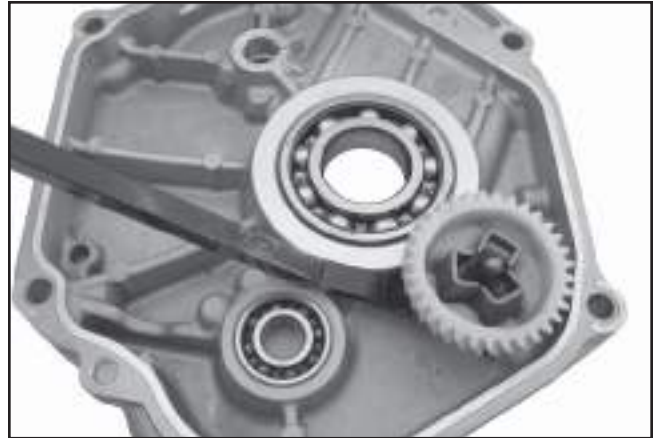
Figure 9-61. Pry Governor Gear to Remove.
