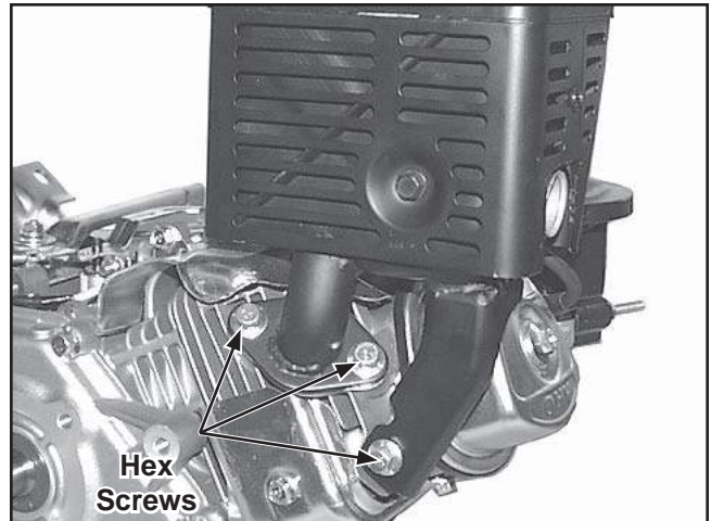
Figure 11-86. Install CH270 Muffler/Heat Shield Assembly.
