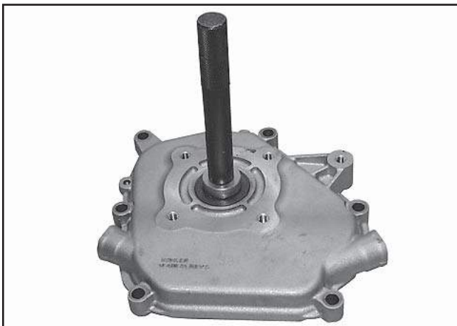
Figure 11-4. Install Closure Plate Oil Seal.
