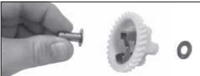
Figure 9-59. CH395 Governor Assembly Components.
