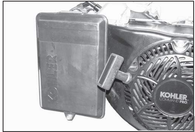
Figure 4-6. Low-Profile Air Cleaner.
