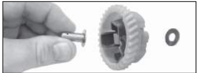
Figure 9-62. CH440 Governor Assembly Components.
