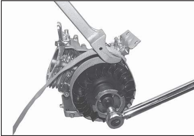
Figure 11-40. Torque Flywheel Nut.
