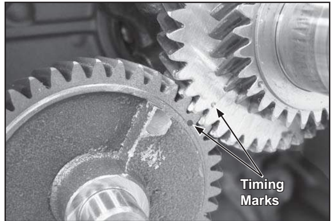
Figure 11-27. Aligning Timing Marks.
