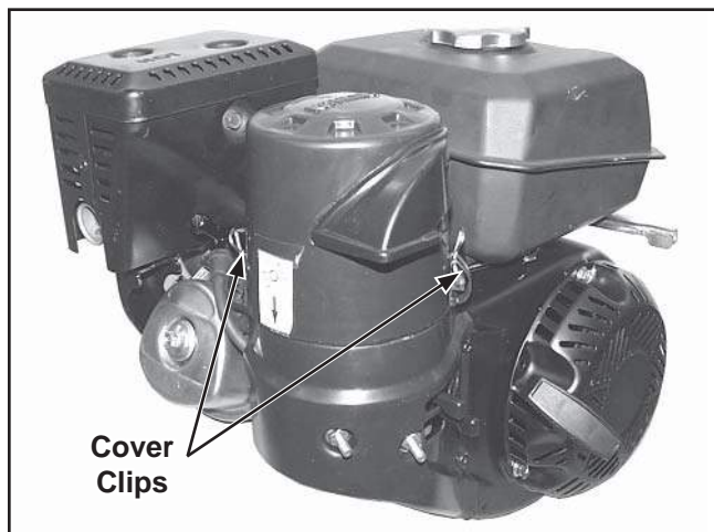
Figure 11-90. Install Air Cleaner Cover.
