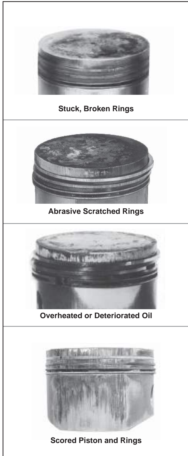
Figure 10-12. Common Types of Piston Damage.
