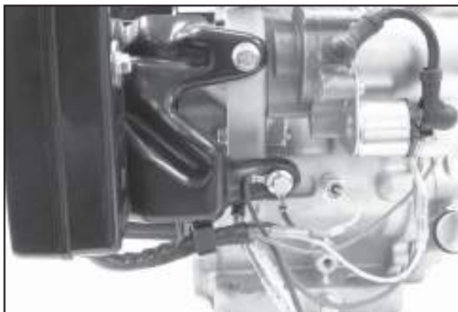
Figure 11-69. Mount and Torque Control Panel Hex Flange Screws.
