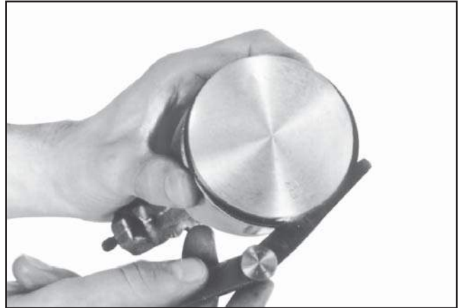
Figure 10-14. Measuring Piston Ring Side Clearance.
