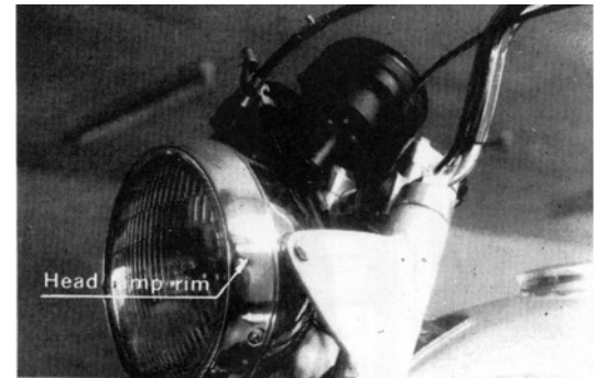
Fig. 95 Removing headlight rim
