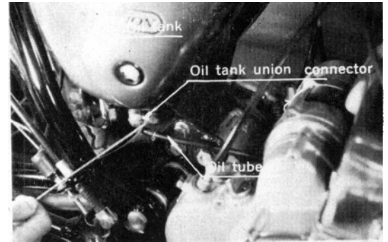
Fig. 4 Disconnecting oil tube C
