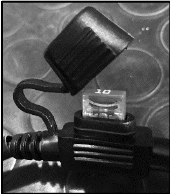
Harness fuse and its holder opened
