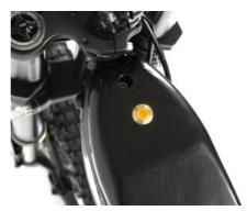
65% and red when the battery charge reaches 30%. The red light will start blinking when the battery charge is very low. From this point, the bike will start losing power and will be able to travel roughly 2-3 km (1-2 miles) before the motorcycle shuts down completely.
