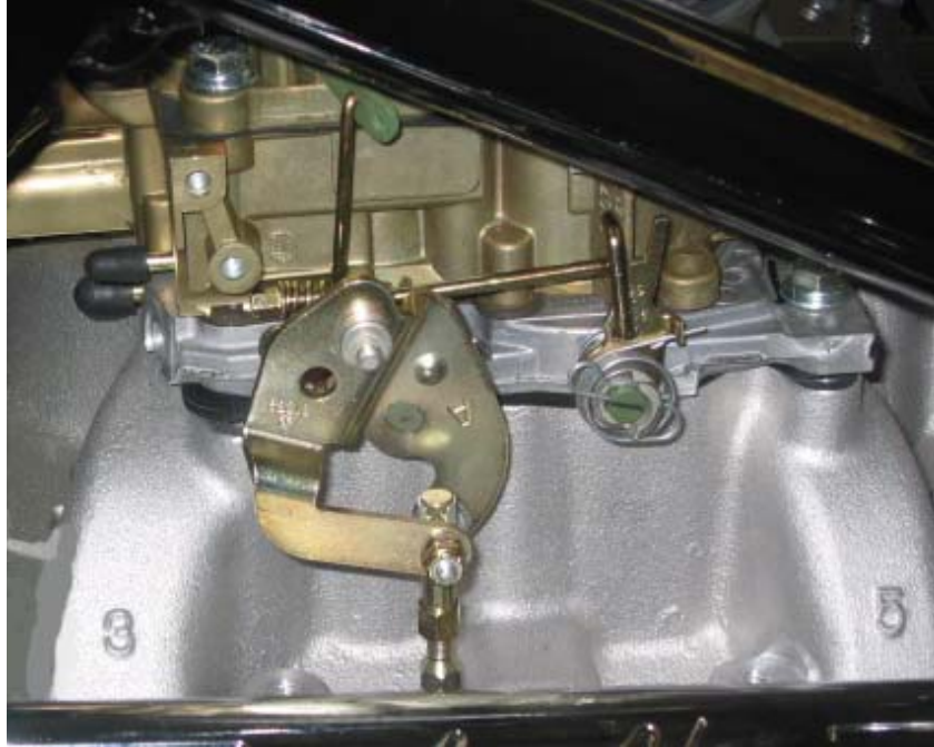
Throttle Linkage Connection at Carburetor Fig. 5-3
