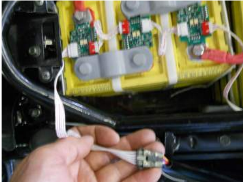
This string ends in a connector to the black wire coming out of the BMS box.
