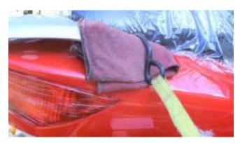
Place one strap on each side of the bike on the swing arm rear by the shock pulling backward at least 45 degrees or more. This is to prevent the bike from moving forward on braking of the transport vehicle.
