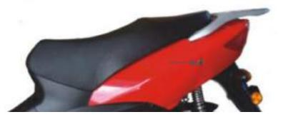
Push down on the seat while turning the lock. Do not let the seat fly up or it may cause damage.
