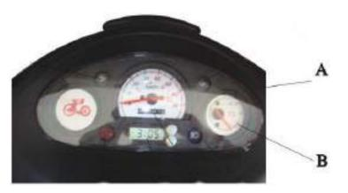
Power Meter – On the right side of the instrument panel (A) is a power gauge (B). Only when the needle is at the top of the arc is the bike charged for good road use. When it enters the broad band arc areas the bike is in danger of running out of power. When it reaches the bottom arc it will shut off to protect itself. A clock is in the center bottom and can be set by the two buttons to the right.
