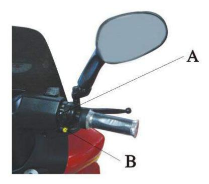
Switch B is a switch to raise or lower the amperage and volts that the motor gets. There are three positions. Use the lowest power setting that you can to maintain the desired speed. You will feel the difference when pushing the button.
