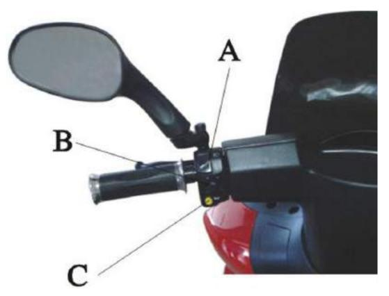
On the left handgrip is a rocker switch for high and low beam. Switch A
