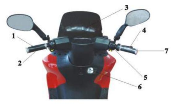
The power on key and steering lock is shown as (6) in the above photo.
